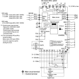
(Note) Noise filter is installed in 200V 0.4~7.5kW, 400V 0.75~15kW
