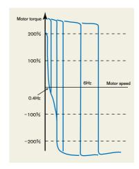
Example torque characteristics of VFA7-2037PL with a 4P-3.7kw stardard motor.
